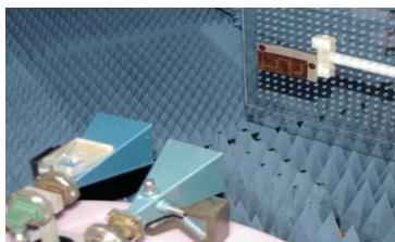
Fig.4 Experimental set up of chipless tag in anechoic chamber
