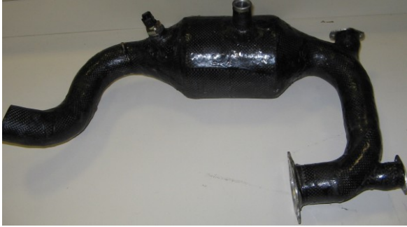
Carbon Fibre Intake Manifold
